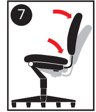
7 Mid-Range Knee Tilt Pivot point located slightly ahead of center of chair base. Allows user to recline at a slightly more relaxed angle than conventional tilt.
