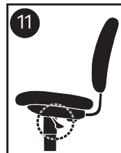
11 Tilt Lock Locks out tilt function when chair is in upright position.
