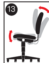
13 Multi-Task Control Adjusts seat and back angles with a single lever (infinite locking within a fixed range).
