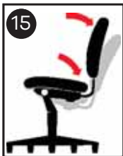
15 Synchronized Knee Tilt Back reclines at a 2-to-1 ratio to seat angle. Pivot point located near front edge of chair.
